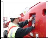
**The operator** performs visual and function checks to identify faults before use.
